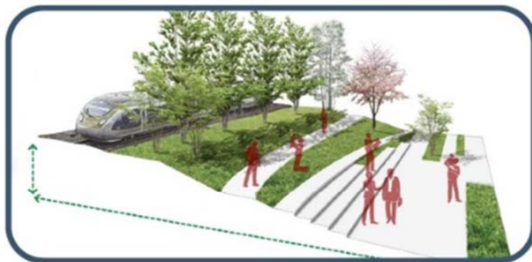
This drawing depicts a proposed terraced levee system for raising the railroad tracks to limit increased risk of flooding due to sea level rise.
