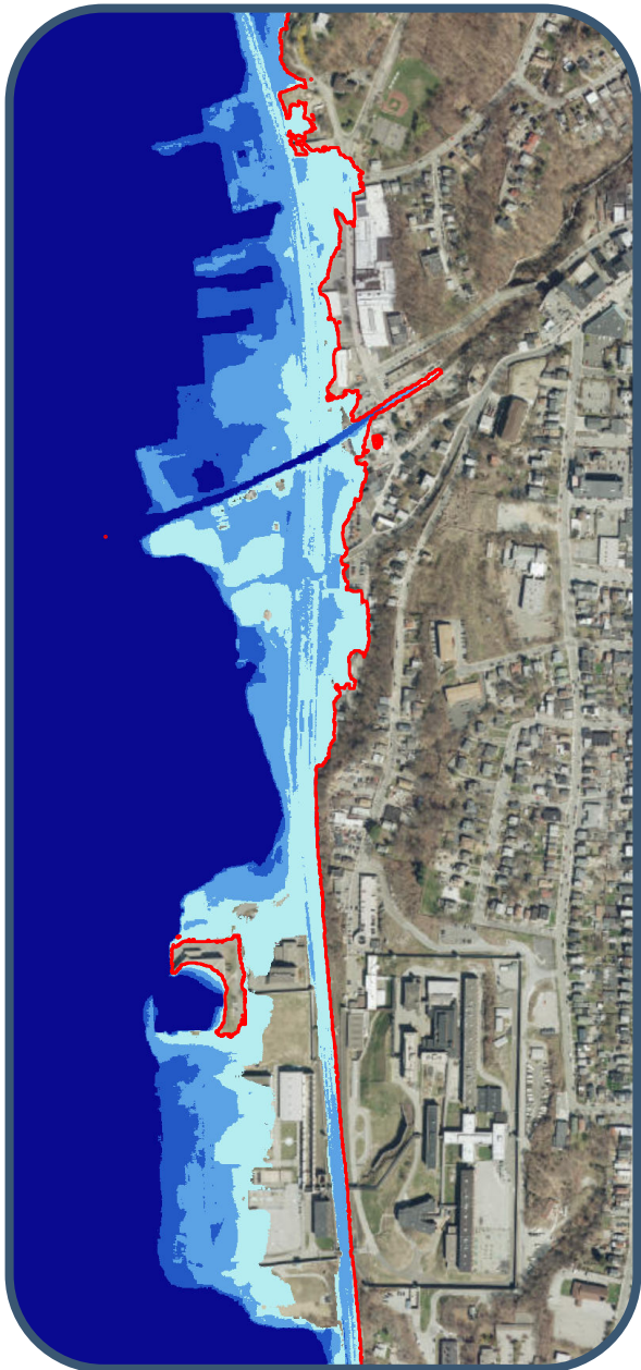
Depths of temporary flooding anticipated in the “100-year” or 1% flood zone on the Ossining waterfront for the present-day baseline condition.
