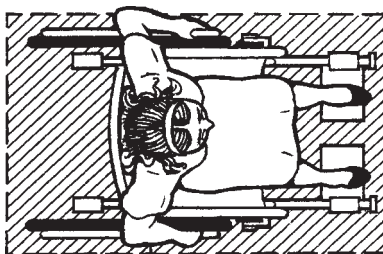
Clear Floor Space for Wheelchair Parking at Appliances and Fixtures
